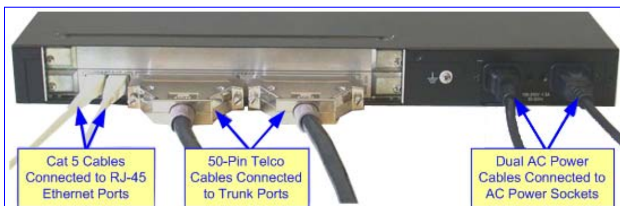
Figure 2-6: Rear-Panel Cabling for 16 Trunks (Dual AC)
