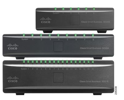
**System LED—**(Green) This LED lights up and remains lit when the switch is powered on.
