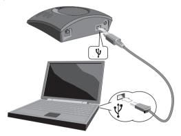
Figure 2 - Connecting to a PC
