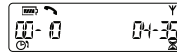
Elapsed call time (left) and remaining talk time (right) are shown during a call
