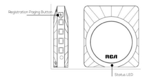
The registration/paging button is located on the right hand side of the gateway. When the gateway is powered up, the status LED will be on and amber colored for 5 seconds. After the initialization, the LED status indicators are as follows:
