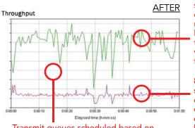
Transmit queues scheduled based on the airtime constraints per station using weighted round robin algorithm 802.11n stations experience much higher levels of throughput with airtime fairness
