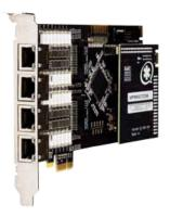
Digium Wildcard TE820 PCI Express ISDN PRI Card (1TE820F) card supports industry standard telephony protocols, including multiple variants of Primary Rate ISDN. Each span can be configured as either CPE or network for optimal flexibility. The optional VPMOCT256 hardware echo cancellation module, based on the industry-leading Octasic chipset, offloads the task of echo
