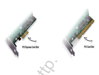
OpenVox AE1610E takes full advantage of Octasic® Hardware Echo Cancellation Module to deliver the superior voice quality on both FXO and FXS interfaces in all 16 ports. AE1610E is a new generation analog card with Octasic® Hardware Echo Cancellation Module on board. With the interchangeable quad-FXS and quad-FXO modules, AE1610E can eliminate the requirement for separate channel banks or access gateways. OpenVox A1610E03 Highlights
