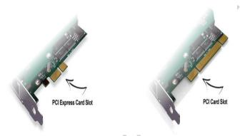
The OpenVox B200E PCI Express ISDN BRI Card is a PCI Express 2.2 compliant card supporting 2 BRI S/T interfaces, with a onboard multi NT powerfeeding circuit . NT/TE mode can be independently configured on each of the 2 ports.
