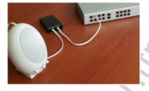
Rapid PA connected to Astribank and loudspeaker with internal amplifier
