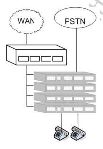
System architecture illustrating XR3000 connected to WAN and additional Astribank units via USB.
