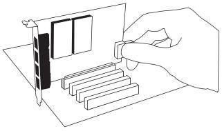
Figure 6: Connect Power for FXS Modules
