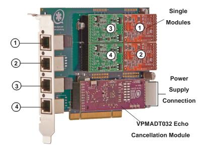
Figure 2: TDM410 Card with Four Single Modules
