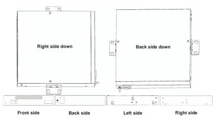
Figure 6: Acceptable Wall Mount Orientations
