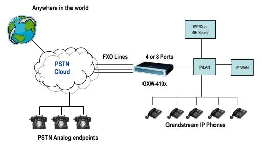
FIGURE 3: FUNCTIONAL DIAGRAM OF IP-PBX & GXW410X
