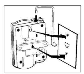
Fig. 6 - Wall mounting installation.
