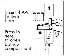
Fig. 7 - Battery installation
