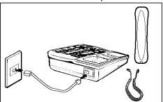
Fig.3 - Connections and installation
