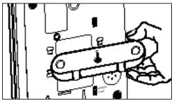
Fig. 5 - Phone base installation for wall mounting
