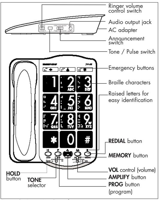
Figure 2 - Base Unit Controls
