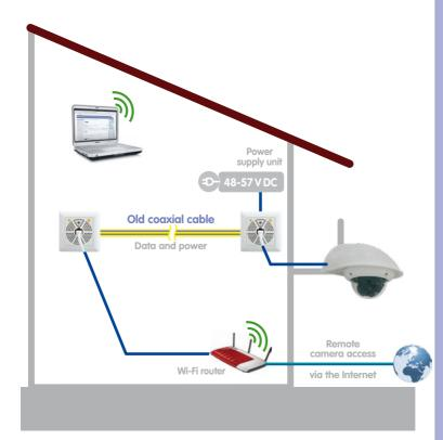
Only the analog camera needs to be replaced with a HiRes camera. The coaxial cable and potentially even the analog camera's power supply unit can still be used
