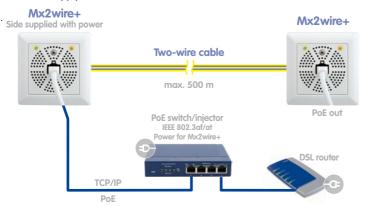
By default, Mx2wire+ logs onto the switch as a PoE class 0 device (can be changed to class 4).
