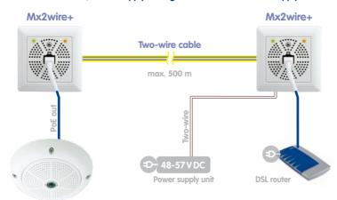
The power required for Mx2wire+ and one PoE end device can be supplied by connecting an external power supply unit (48–57 V DC, 600 mA) to another Mx2wire+ unit (max. power output for end device: PoE class 3/13 W). The external power can also be supplied via the unit to which the PoE end device is connected in order to reduce unnecessary performance losses.
