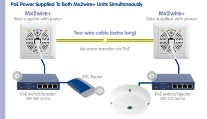
If the two-wire cable is not sufficient to supply the Mx2wire+ remote station with power due to its length, both sides can be supplied with power via PoE.
