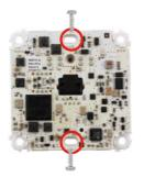
The circuit board is attached directly to the socket using two screws (item 1.4.) (see left) or it is attached to the wall using the Torx screws (see page 24)
