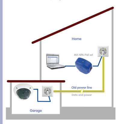
Here, a two-wire cable, formerly used as a power connection, serves to connect an IP camera in a garage while keeping costs to a minimum
