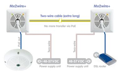
If the two-wire cable is not sufficient to supply the Mx2wire+ remote station with power due to its length, both Mx2wire+ units can be supplied with power via a power supply unit (48–57 V DC, 600 mA).
