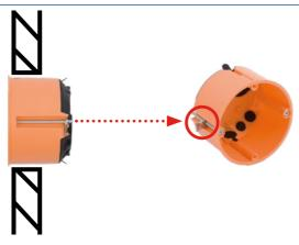
When the screws are tightened, the metal claws automatically pop out and clamp the socket to the cavity wall (made of wood or plasterboard, for example)
