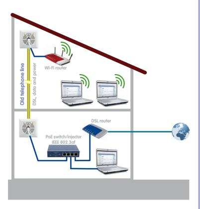
Power is supplied to the Wi-Fi router via the Mx2wire+ devices (max. 13 W)
