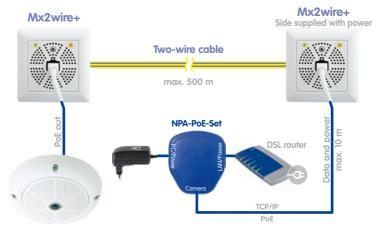
The blue NPA-PoE set, which is available as an accessory from MOBOTIX (MX-NPA-PoE set), can be used as an alternative to the standard PoE switch (IEEE 802.3af).
