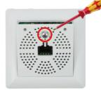
Now remove the attached frame from the circuit board. Please note that you will need the stainless steel screw in the front panel again later.
