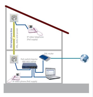
No power connection is required for the Mx2wire+ device and IP telephone as up to 13 watts of power can be supplied via PoE
