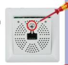
2. Using a small screwdriver, switch the rotary switch on the Mx2wire+ connected to the injector/switch from position 3 to position 4 (see figure). This setting corresponds to the PoE classes 3 and 4 of the injector/ switch used.
