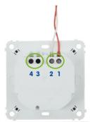
Outputs of power supply unit to screw terminals 3 and 4: If, instead of a PoE switch/injector, a DC power supply unit (48–57 V) is used to supply power, it is connected to one of the two Mx2wire+ units. See the description for alternative connection options in Section 3.2.
