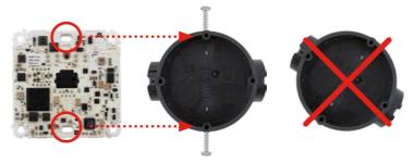
2. Use four or two (diagonally opposite one another) Torx screws/screw anchors (item 1.6) to tightly screw the Mx2wire+ housing and circuit board to the wall. We recommend this procedure if the installed in-wall socket is not properly aligned or is not flush with the wall. Otherwise, the Mx2wire+ unit could easily be pulled out together with the in-wall socket.
