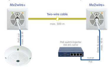
Mx2wire+ requires a PoE power supply via a standard PoE switch (class 0, IEEE 802.3af or class 4, IEEE 802.3at) for operation
