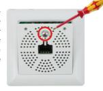
Now remove the attached frame from the circuit board. Please note that you will need the stainless steel screw in the front panel again later.
