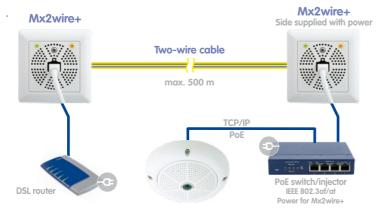
Connecting to the DSL router without a power supply is only possible if PoE power is supplied to the other Mx2wire+ unit.
