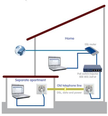
Mx2wire+ eliminates the enormous amount of time and cost normally required for cabling simply by reusing the old telephone line as a network cable
