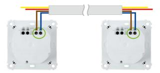
Before installing the two Mx2wire+ units, test the cable connection to ensure that it is functioning properly (if necessary, draw up a test chart). Due to their design, coaxial cables and Ethernet cables (Cat7) are particularly suited for longer distances.
